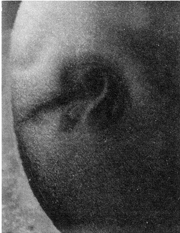
Fig. 3(a) Starting plume moving radially inward, produced by heater shown in Fig. 2; rotor speed 531 rpm
